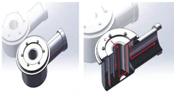
SUPPLEMENTARY FIGURE S4. Model diagram of a bathroom floor drain and schematic diagram of water flow direction of a centralized quarantine apartment in Beijing.
