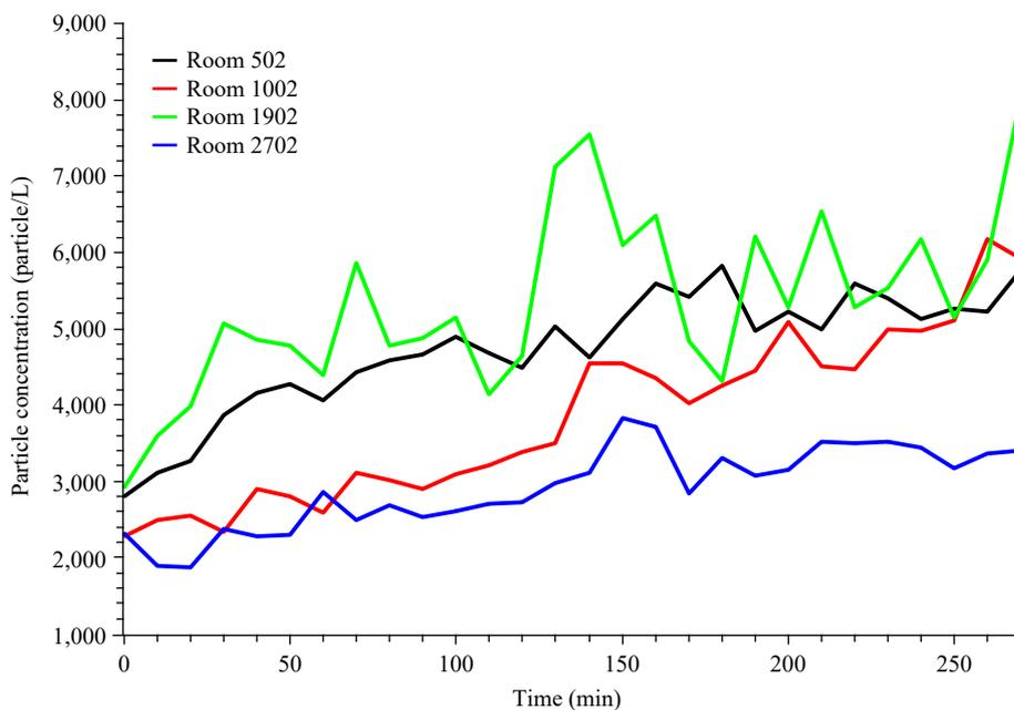
SUPPLEMENTARY FIGURE S3. The changes of particle concentration over time at  $1\ \mu\text{m}$  in 2 scenarios in different rooms. Note: Two scenarios, breathing (scenario 1, 0–130 min) and breathing with defecation with toilet flushing (scenario 2, 140–270 min), were simulated in bathroom 402. Changes in particle number concentrations were monitored in bathrooms 502, 1002, 1902, and 2702.
